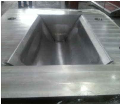
图10 凸凹曲率蒙皮充液成形工装 Fig.10 Hyperbolic skin hydroforming fixture
