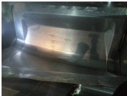
图11 凸凹曲率蒙皮充液成形零件 Fig.11 Hyperbolic skin part after hydroforming process
